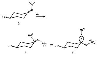
Then MeLi appears to attack the carbonyl carbon of the complex 4 or 4' from the sterically less hindered side leading to the equatorial alcohol 3 in accord with the experimental findings. The initial ate complex formation by the attack of MeLi to the aluminum reagent followed by reaction with the ketone seems to be unlikely, since treatment of 1 with a mixture of MeLi and MAD at -78 °C gave a result (axial/equatorial = 84:16) similar to that in the sole addition of MeLi.
